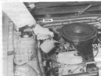
Running oil around the inlet manifold joints to check for air leaks.
